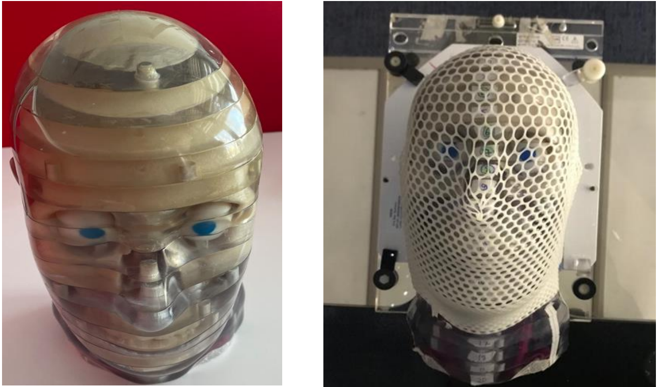
Figure 2. a) Phantom produced by a 3D printer b) Placing a thermoplastic mask on the phantom produced by a 3D printer.
